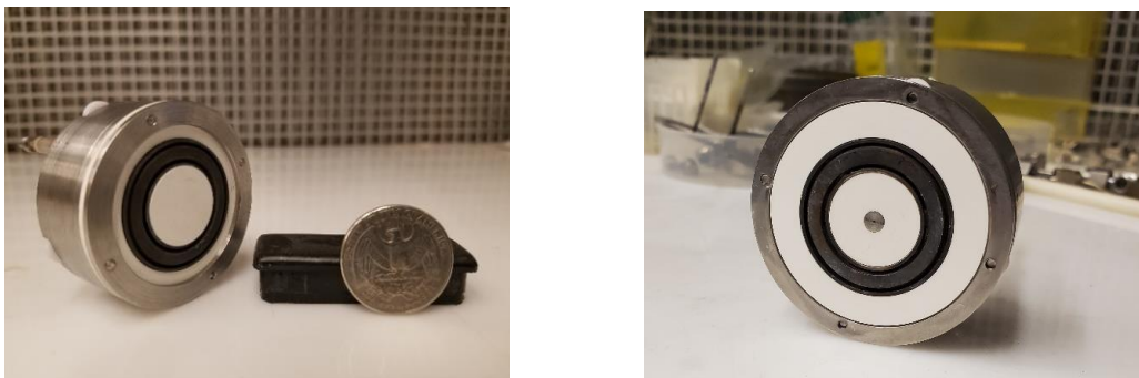
Figure 3. Two variants of wall-less Hall thruster: (left) thruster with Boron Nitride in the center and (right) thruster with a steel gas distributor electrode in the center.
